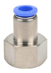
NITRA pneumatic push-to-connect fitting, straight, nickel-plated brass body, nickel-plated brass threads, (1) R3/8 female BSPT to (1) 5/16in (8mm) push-to-connect. Package of 5.
