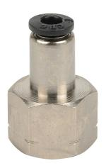
NITRA pneumatic push-to-connect fitting, straight, nickel-plated brass body, nickel-plated brass threads, (1) 1/4in female NPT to (1) 5/32in (4mm) push-to-connect. Package of 5.
