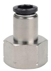
NITRA pneumatic push-to-connect fitting, straight, nickel-plated brass body, nickel-plated brass threads, (1) 3/8in female NPT to (1) 5/16in (8mm) push-to-connect. Package of 5.
