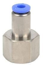
NITRA pneumatic push-to-connect fitting, straight, nickel-plated brass body, nickel-plated brass threads, (1) R1/4 female BSPT to (1) 5/32in (4mm) push-to-connect. Package of 5.
