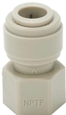
HydroMode potable water push-to-connect fitting, female, straight, acetal body, acetal threads, (1) 3/8in tube to (1) 1/4in female NPT connection(s), NSF/ANSI 61. Package of 5.
