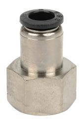
NITRA pneumatic push-to-connect fitting, straight, nickel-plated brass body, nickel-plated brass threads, (1) 1/2in female NPT to (1) 3/8in push-to-connect. Package of 5.
