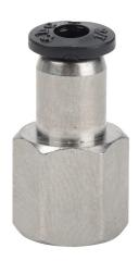
NITRA pneumatic push-to-connect fitting, straight, nickel-plated brass body, nickel-plated brass threads, (1) 1/8in female NPT to (1) 1/8in push-to-connect. Package of 5.
