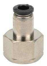
NITRA pneumatic push-to-connect fitting, straight, nickel-plated brass body, nickel-plated brass threads, (1) 3/8in female NPT to (1) 1/4in push-to-connect. Package of 5.
