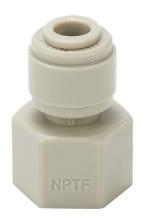
HydroMode potable water push-to-connect fitting, female, straight, acetal body, acetal threads, (1) 1/4in tube to (1) 1/4in female NPT connection(s), NSF/ANSI 61. Package of 5.
