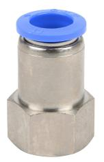
NITRA pneumatic push-to-connect fitting, straight, nickel-plated brass body, nickel-plated brass threads, (1) R3/8 female BSPT to (1) 12mm push-to-connect. Package of 5.
