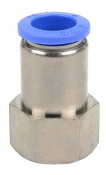
NITRA pneumatic push-to-connect fitting, straight, nickel-plated brass body, nickel-plated brass threads, (1) R1/4 female BSPT to (1) 12mm push-to-connect. Package of 5.
