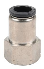
NITRA pneumatic push-to-connect fitting, straight, nickel-plated brass body, nickel-plated brass threads, (1) 1/2in female NPT to (1) 1/2in push-to-connect. Package of 5.
