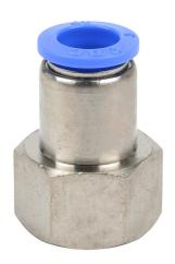
NITRA pneumatic push-to-connect fitting, straight, nickel-plated brass body, nickel-plated brass threads, (1) R3/8 female BSPT to (1) 10mm push-to-connect. Package of 5.
