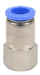
NITRA pneumatic push-to-connect fitting, straight, nickel-plated brass body, nickel-plated brass threads, (1) R1/4 female BSPT to (1) 10mm push-to-connect. Package of 5.
