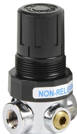
HydroMode miniature potable water pressure regulator, 1/8in female NPT inlet(s), 1/8in female NPT outlet(s), 0-100 psi adjustable range, suitable for potable water applications.
