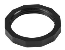
HydroMode panel nut, 1-3/16-18 UNEF threads. For use with FR-8 series water regulators.
