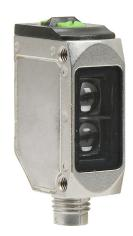
AutomationDirect photoelectric sensor, rectangular, 316L stainless steel, diffuse with background suppression, 200mm sensing distance, selectable light-on/dark-on, PNP, potentiometer, 1 kHz switching frequency, 4-pin M8 quick-disconnect.
