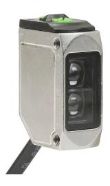
AutomationDirect photoelectric sensor, rectangular, 316L stainless steel, diffuse with background suppression, 200mm sensing distance, selectable light-on/dark-on, PNP, potentiometer, 1 kHz switching frequency, 4-pin M12 quick-disconnect.
