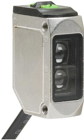
AutomationDirect photoelectric sensor, rectangular, 316L stainless steel, diffuse with background suppression, 200mm sensing distance, selectable light-on/dark-on, PNP, potentiometer, 1 kHz switching frequency, 4-pin M12 quick-disconnect.
