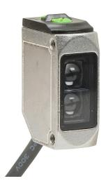
AutomationDirect photoelectric sensor, rectangular, 316L stainless steel, diffuse with background suppression, 200mm sensing distance, selectable light-on/dark-on, PNP, potentiometer, 1 kHz switching frequency, 6.5ft/2m cable length, pigtail.
