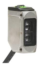
AutomationDirect photoelectric sensor, rectangular, 316L stainless steel, diffuse with background suppression, 200mm sensing distance, selectable light-on/dark-on, NPN, potentiometer, 1 kHz switching frequency, 4-pin M12 quick-disconnect.
