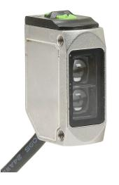
AutomationDirect photoelectric sensor, rectangular, 316L stainless steel, diffuse with background suppression, 200mm sensing distance, selectable light-on/dark-on, NPN, potentiometer, 1 kHz switching frequency, 6.5ft/2m cable length, pigtail.
