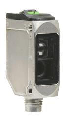
AutomationDirect photoelectric sensor, rectangular, 316L stainless steel housing, through-beam receiver, 10m sensing distance, 10-30 VDC operating voltage, selectable light-on/dark-on, PNP, 3-wire, 4-pin M8 quick-disconnect.
