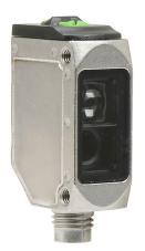
AutomationDirect photoelectric sensor, rectangular, 316L stainless steel housing, through-beam receiver, 10m sensing distance, 10-30 VDC operating voltage, selectable light-on/darkon, PNP, 3-wire, 4-pin M8 quick-disconnect.
