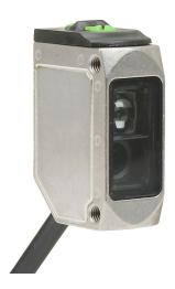
AutomationDirect photoelectric sensor, rectangular, 316L stainless steel housing, through-beam receiver, 10m sensing distance, 10-30 VDC operating voltage, selectable light-on/dark-on, PNP, 3-wire, 4-pin M12 quick-disconnect.
