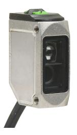
AutomationDirect photoelectric sensor, rectangular, 316L stainless steel housing, through-beam receiver, 10m sensing distance, 10-30 VDC operating voltage, selectable light-on/darkon, PNP, 3-wire, pigtail.
