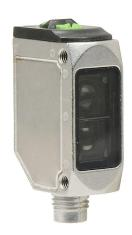
AutomationDirect photoelectric sensor, rectangular, polarized retroreflective, visible red, 5m sensing distance, selectable light-on/dark-on, PNP, potentiometer, 3-wire, 4-pin M8 quick-disconnect.
