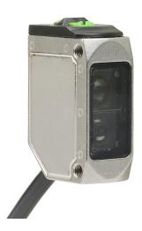
AutomationDirect photoelectric sensor, rectangular, polarized retroreflective, visible red, 5m sensing distance, selectable light-on/dark-on, PNP, potentiometer, 3-wire, 4-pin M12 quick-disconnect.
