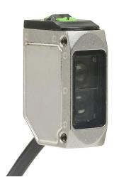
AutomationDirect photoelectric sensor, rectangular, polarized retroreflective, visible red light emission, 5m sensing distance, selectable light-on/dark-on, PNP, potentiometer, 3-wire, 4-pin M12 quick-disconnect.
