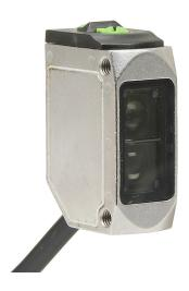
AutomationDirect photoelectric sensor, rectangular, polarized retroreflective, visible red, 5m sensing distance, selectable light-on/dark-on, PNP, potentiometer, 3-wire, pigtail.
