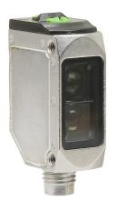
AutomationDirect photoelectric sensor, rectangular, polarized retroreflective, visible red, 5m sensing distance, selectable light-on/dark-on, NPN, potentiometer, 3-wire, 4-pin M8 quick-disconnect.
