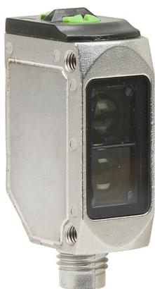
AutomationDirect photoelectric sensor, rectangular, polarized retroreflective, visible red, 5m sensing distance, selectable light-on/dark-on, NPN, potentiometer, 3-wire, 4-pin M8 quick-disconnect.
