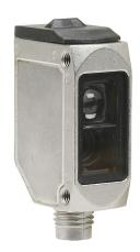
AutomationDirect photoelectric sensor, rectangular, 316L stainless steel housing, through-beam emitter, visible red light emission, 10m sensing distance, 10-30 VDC operating voltage, 3-wire, 4-pin M8 quick-disconnect.
