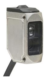
AutomationDirect photoelectric sensor, rectangular, 316L stainless steel housing, through-beam emitter, visible red, 10m sensing distance, 10-30 VDC operating voltage, 3-wire, 4-pin M12 quick-disconnect.
