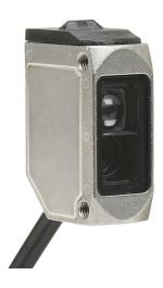
AutomationDirect photoelectric sensor, rectangular, 316L stainless steel housing, through-beam emitter, visible red, 10m sensing distance, 10-30 VDC operating voltage, 3-wire, pigtail.
