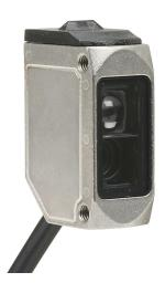
AutomationDirect photoelectric sensor, rectangular, 316L stainless steel housing, through-beam emitter, visible red light emission, 10m sensing distance, 10-30 VDC operating voltage, 3-wire, pigtail.
