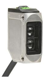
AutomationDirect photoelectric sensor, rectangular, diffuse, visible red, 500mm sensing distance, selectable light-on/dark-on, PNP, potentiometer, 1 kHz switching frequency, 316L stainless steel housing, 4-pin M12 quick-disconnect.
