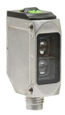
AutomationDirect photoelectric sensor, rectangular, diffuse, visible red, 500mm sensing distance, selectable light-on/dark-on, NPN, potentiometer, 1 kHz switching frequency, 316L stainless steel housing, 4-pin M8 quick-disconnect.
