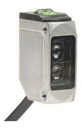
AutomationDirect photoelectric sensor, rectangular, diffuse, visible red, 500mm sensing distance, selectable light-on/dark-on, NPN, potentiometer, 1 kHz switching frequency, 316L stainless steel housing, 4-pin M12 quick-disconnect.
