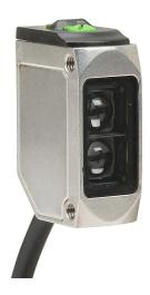
AutomationDirect photoelectric sensor, rectangular, diffuse, visible red, 500mm sensing distance, selectable light-on/dark-on, NPN, potentiometer, 1 kHz switching frequency, 316L stainless steel housing, pigtail.
