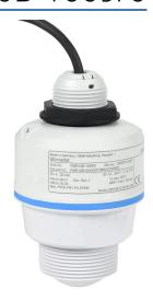
Endress+Hauser Micropilot frequency modulated continuous wave (FMCW) radar liquid or bulk solids level sensor, 32.8ft/10m sensing range, 4–20 mA, 12–30 VDC, 1-1/2in male NPT process connection.
