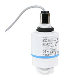
Endress+Hauser Micropilot pulsed radar liquid level sensor, 26.2ft/8m or 39.3ft/12m with flooding protection tube sensing range, 4-20 mA, 10.5-30 VDC operating voltage, 1-1/2in male NPT process connection.
