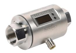
ProSense liquid flow meter, magnetic-inductive, 3/4 inch female NPT process connection, 0 to 13.2 GPM, -4 to 176 F, 0.01 to 30,000,000 Gallons, Output: switch or pulse, Output 2: switch, analog or reset input, 19 to 30 VDC operating voltage.
