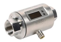
ProSense liquid flow meter, magnetic-inductive, 3/4in female NPT process connection, 0 to 13.2 GPM, -4 to 176 deg F, 0.01 to 30,000,000 gallons, Output: switch or pulse, Output 2: switch, analog or reset input.
