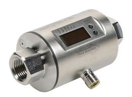
ProSense liquid flow meter, magnetic-inductive, 1/2in female NPT process connection, 0 to 6.6 GPM, -4 to 176 F, Output: analog, Output 2: analog, 20 to 30 VDC operating voltage.
