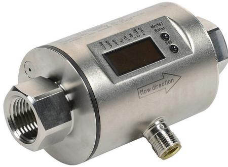
ProSense liquid flow meter, magnetic-inductive, 1/2in female NPT process connection, 0 to 6.6 GPM, -4 to 176 deg F, 0.01 to 30,000,000 gallons, Output: switch or pulse, Output 2: switch, analog or reset input.
