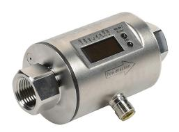
ProSense liquid flow meter, magnetic-inductive, 1/2in female NPT process connection, 0 to 6.6 GPM, -4 to 176 F, 0.01 to 30,000,000 Gallons, Output: switch or pulse, Output 2: switch, analog or reset input, 19 to 30 VDC operating voltage.
