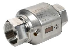
ProSense liquid flow meter, magnetic-inductive, 2in female NPT process connection, 0 to 160 GPM, -4 to 176 deg F, 0.02 to 80,000,000 gallons, Output: switch, pulse or frequency, Output 2: switch, analog or reset input.
