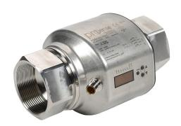
ProSense liquid flow meter, magnetic-inductive, 2in female NPT process connection, 0 to 160 GPM, -4 to 176 F, 0.02 to 80,000,000 Gallons, Output: switch, pulse or frequency, Output 2: switch, analog or reset input, 18 to 32 VDC operating voltage.
