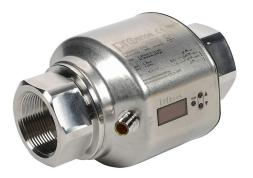
ProSense liquid flow meter, magnetic-inductive, 1-1/2in female NPT process connection, 0 to 79.3 GPM, -4 to 176 deg F, Output: analog, Output 2: analog.
