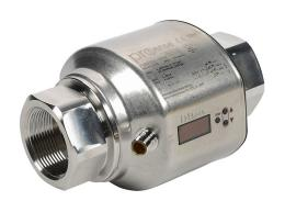
ProSense liquid flow meter, magnetic-inductive, 1-1/2in female NPT process connection, 0 to 79.3 GPM, -4 to 176 F, Output: analog, Output 2: analog, 18 to 32 VDC operating voltage.
