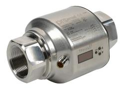
ProSense liquid flow meter, magnetic-inductive, 1-1/2in female NPT process connection, 0 to 80 GPM, -4 to 176 deg F, 0.02 to 80,000,000 gallons, Output: switch, pulse or frequency, Output 2: switch, analog or reset input.
