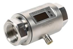
ProSense liquid flow meter, magnetic-inductive, 1in female NPT process connection, 0 to 26.4 GPM, -4 to 176 deg F, 0.01 to 30,000,000 gallons, Output: switch or pulse, Output 2: switch, analog or reset input.
