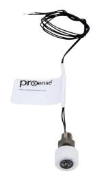
ProSense float liquid level switch, vertical top mount, 0.75in insertion length, 0.78in diameter float, polypropylene, 316 stainless steel wetted parts, -40 to 221 deg F, 1/8in male NPT process connection, SPST reed switch, N.C.
