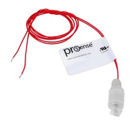
ProSense float liquid level switch, vertical top mount, 1.25in insertion length, 0.59in diameter float, polypropylene wetted parts, -40 to 221 deg F, 1/8in male NPT process connection, SPST reed switch, N.O.
