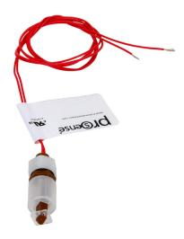
ProSense float liquid level switch, vertical top mount, 1.25in insertion length, 0.59in diameter float, polypropylene wetted parts, -40 to 221 deg F, 3/8-16 male UNC process connection, SPST reed switch, N.O.
