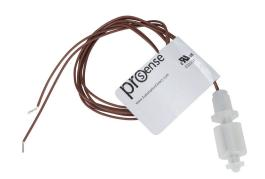
ProSense float liquid level switch, vertical top mount, 1.25in insertion length, 0.58in diameter float, polypropylene wetted parts, -40 to 221 deg F, 1/8in male NPT process connection, SPST reed switch, N.C.
