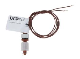
ProSense float liquid level switch, vertical top mount, 1.25in insertion length, 0.58in diameter float, polypropylene wetted parts, -40 to 221 deg F, 3/8-16 male UNC process connection, SPST reed switch, N.C.
