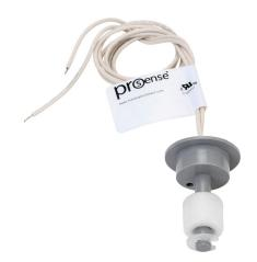
ProSense float liquid level switch, vertical top mount, 1.99in insertion length, 0.875in diameter float, polypropylene wetted parts, -40 to 140 deg F, 3/4in PVC pipe insert process connection, SPST reed switch, N.C.
